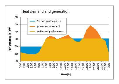
This daily load curve shows a typical output requirement distributed over one day. To cover the highest peaks, you need to install a heat generator that can cover the output peaks.
